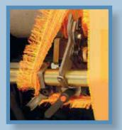
▶ A comprehensive range of electronically controlled devices, such as lateral and central scissors, independent selvedge formation devices, mean setup and changing style is easy and cost-effective.
